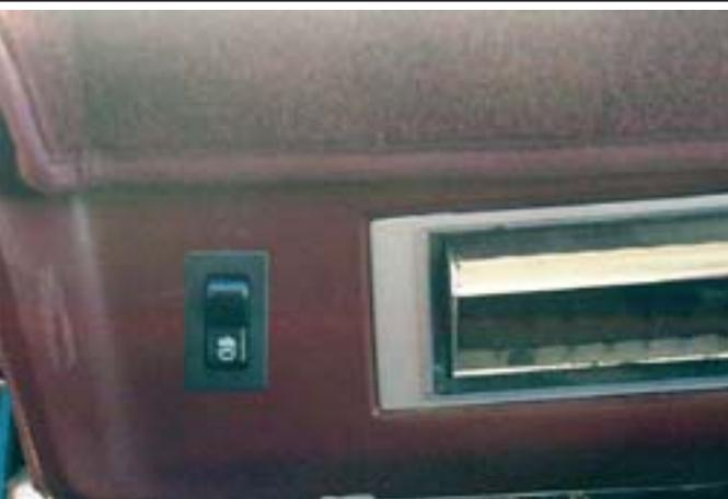
**Step 5-** The switch included with the wiring kit is an inline switch, which will just interrupt power to the relay, so you will have one wire to run to a 12 Volt Positive (+) source, and one to run back to the relay. Cut a hole in your dash by tracing the profile of the switch, or measuring the dimensions, then transferring the template to your dash. The switch just slides into place and locks itself down.
