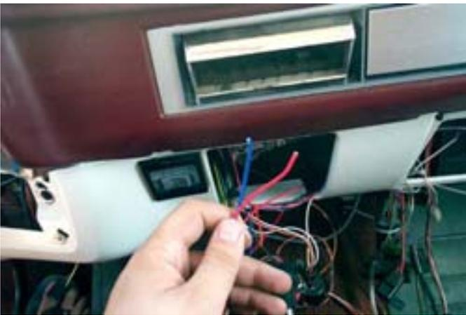
**Step 4-** Decide where you want to put the switch for your lights. Run the Blue wire off of the wiring harness to the Black wire on the switch. The Red wire can be run to any 12 Volt Positive source in your vehicle, since it's only being used as a signal wire, not a power draw. The switch will light up when it is switched to the "on" position.
