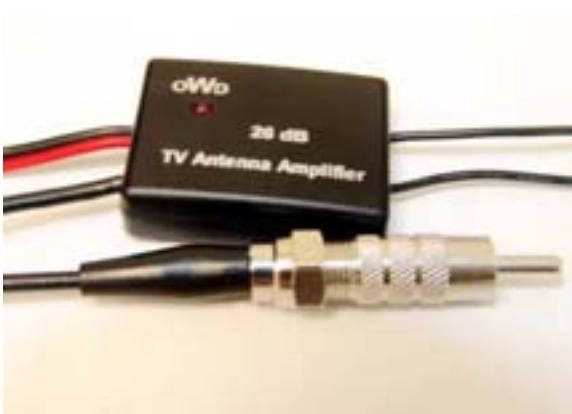
The antenna comes with a co-axial connector with an adapter for european equipment.
