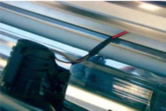
**Step 3-** Attach the wiring harness to the relay and get ready to pull wires. You should already have your lights mounted, so run the pair of Black and Red power wires out to wherever your lights are mounted. You can use a permanent connection by soldering or twisting the wires together and wrapping them in duct tape, or you can use a quick disconnect adapter in case you need to swap them around later.
