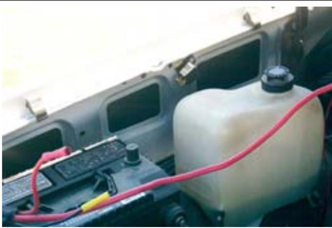
**Step 2-** Once your lights are physically mounted to your vehicle, find a spot close to your battery to mount the relay for the lights. If you use self-tapping metal screws, you won't need to drill any holes. Make sure the relay is accessible to your hands, as you will have to plug it into the wiring harness later.
