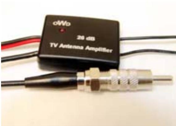
*The antenna comes with a co-axial connector with an adapter for european equipment.*
