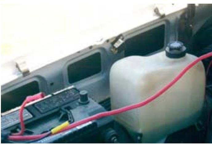
**Step 2-** Once your lights are physically mounted to your vehicle, find a spot close to your battery to mount the relay for the lights. If you use self-tapping metal screws, you won't need to drill any holes. Make sure the relay is accessible to your hands, as you will have to plug it into the wiring harness later.
